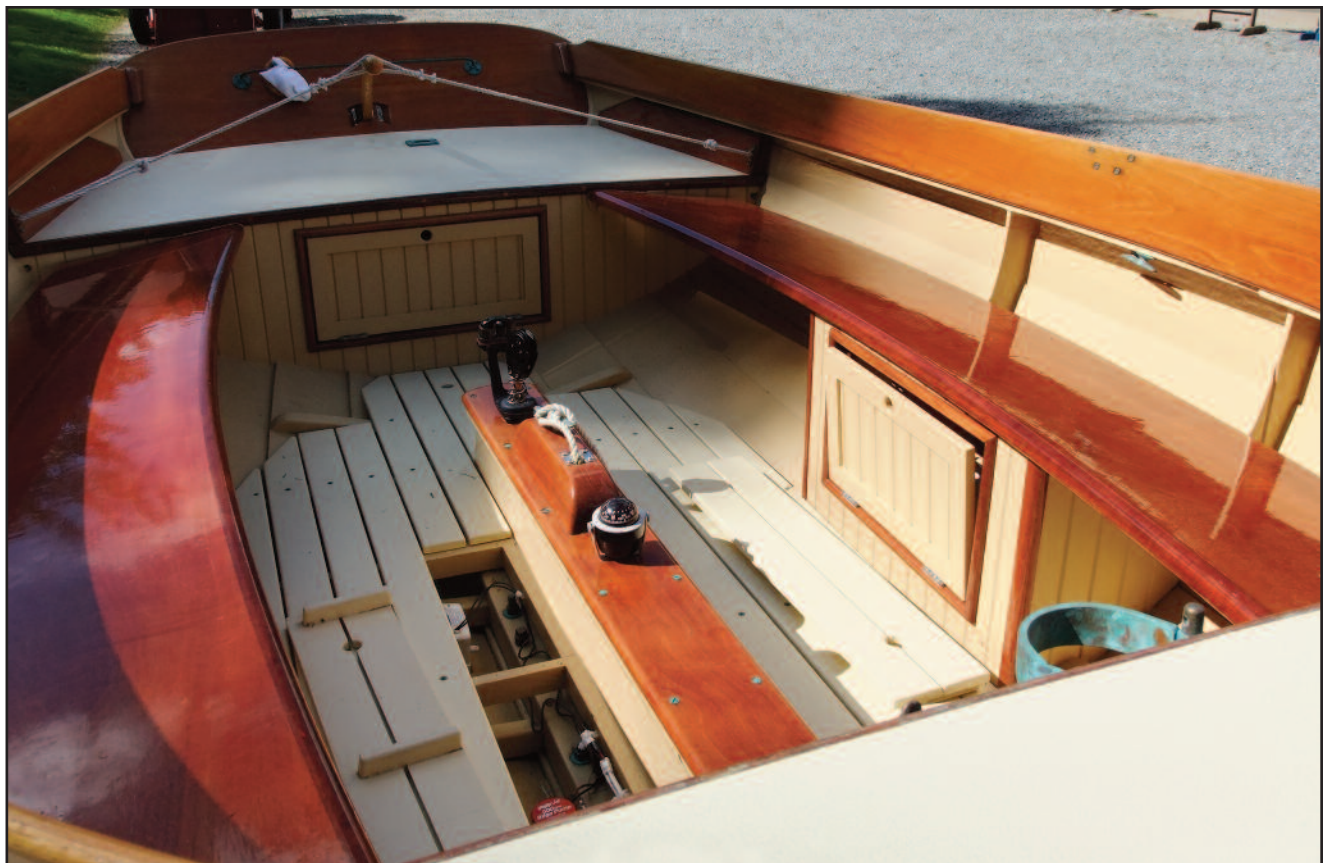
Looking aft in Red Sky hs, showing the handy seat lockers, as well as joinery details of the doors and comfortable angles of the seats and coamings. A couple of the floorboard hatches have been lifted out, showing the floors; trunk log construction; keel bolts; and plenty of room for a bilge pump and float switch.
