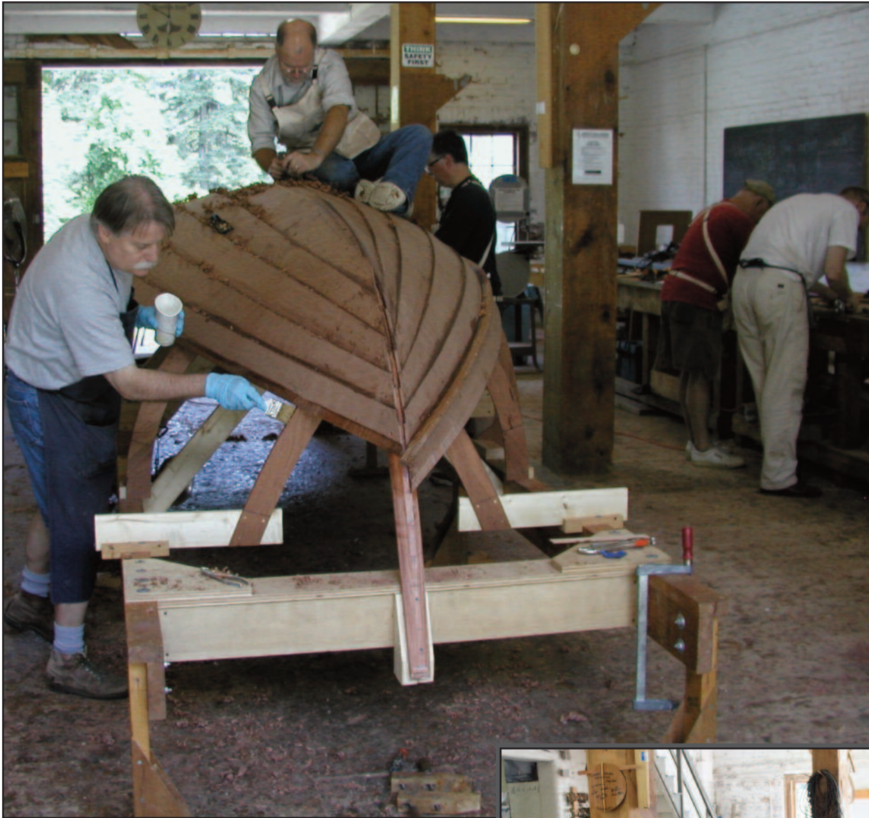
Above: Planking the hull of a Somes Sound 12 1/2 at the WoodenBoat School, Summer 2008.
