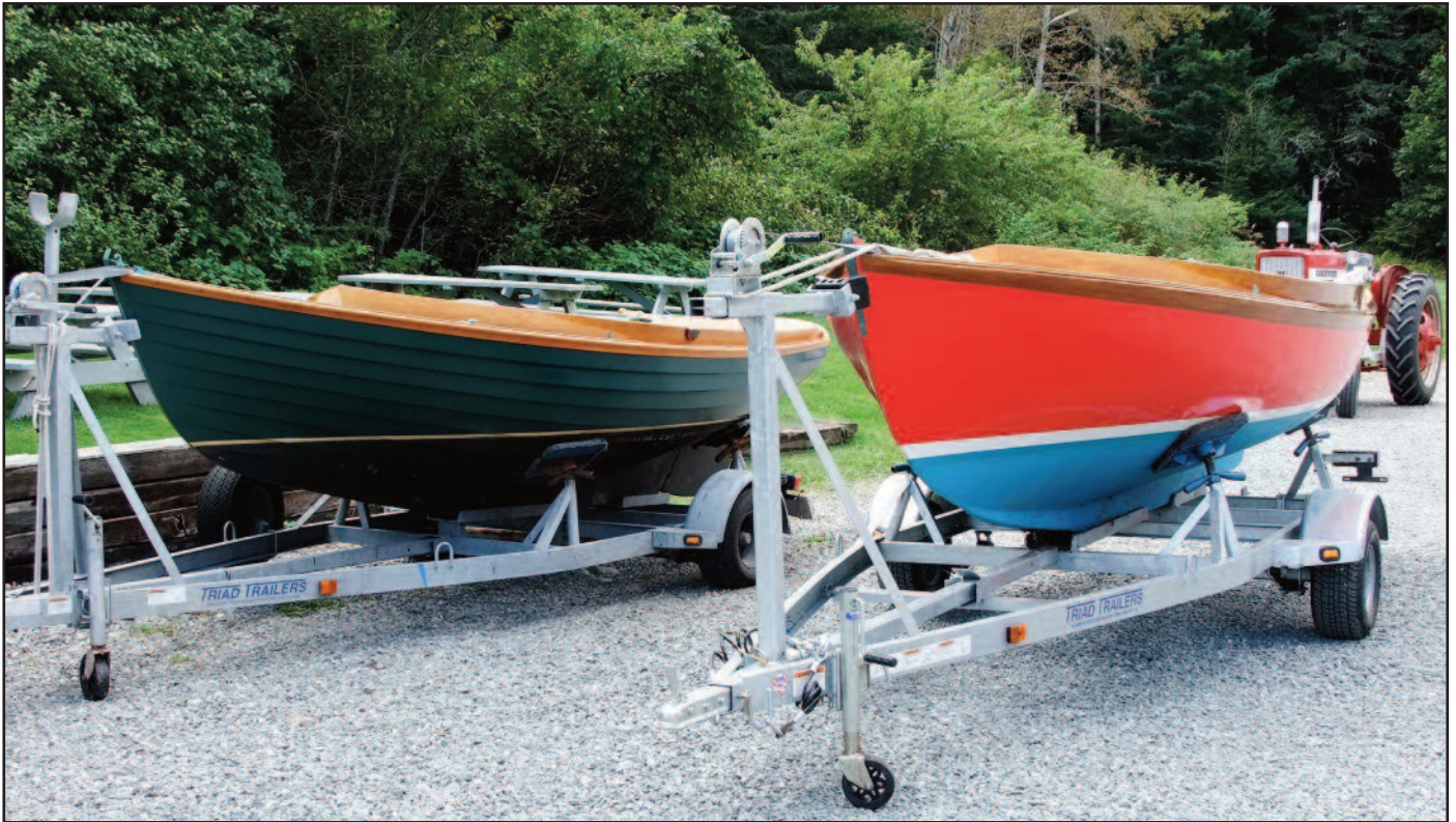
Another look at the Somes Sound 12-1/2 (left) and Haven 12-1/2 together at the end of summer. The Somes Sound 12-1/2's L. Francis Herreshoff-styled stem, shaped rail, and tapered coaming complement each other nicely.
